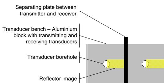
**Example:** Reflector image on the transducer bench at a limit distance for a horizontal triangulation triangle formed to the left.
