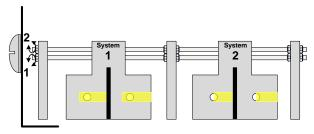
**Example:** Reflector image on the transducer bench at limit distance for horizontal triangulation triangles formed to the left.
