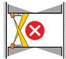
Fig.: 4.5.1-5: Wrong arrangement
