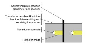
**Example:** Reflector image on the transducer bench at a limit distance for a horizontal triangulation triangle formed to the left.
