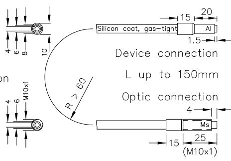
Fibre-optic cable GFKxySI
